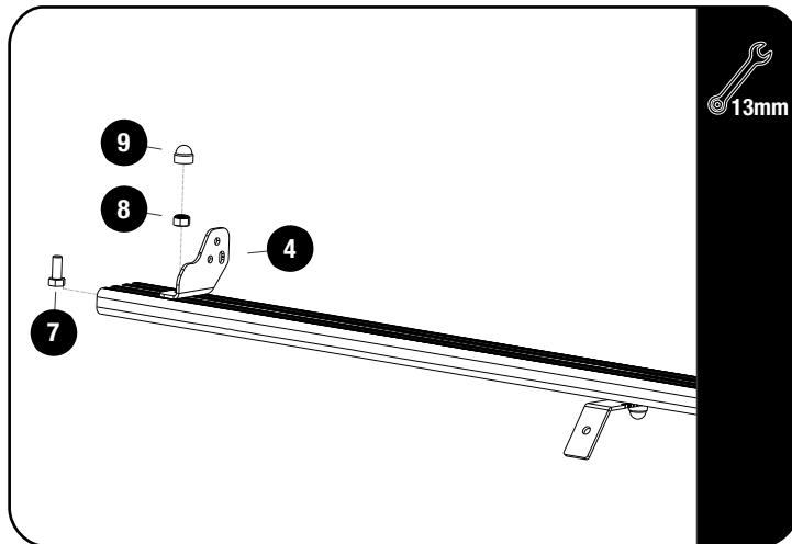
Fit the Light Bar Bracket 01 LH / RH (Item 4) for the 40" Light Bar, using M8x16 Hex Bolt & M8 Nyloc Nut (Items 7 & 8). Fit the light bar and center it on the slat before fully tightening the brackets.
