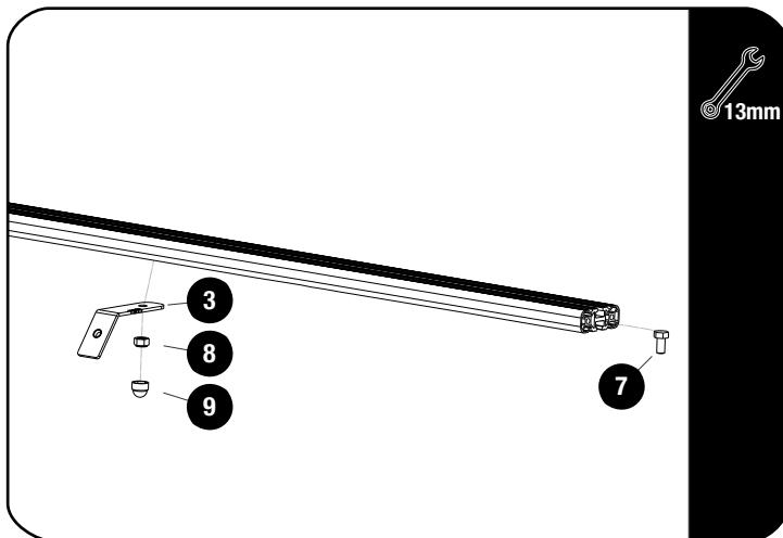
Slide one M8 x 16 Hex Head Bolt (Item 7) into the T-slot of the front slat. Center the mid support bracket in the middle of the slat and secure using M8 Nyloc Nut (Item 8). Fully tighten.
