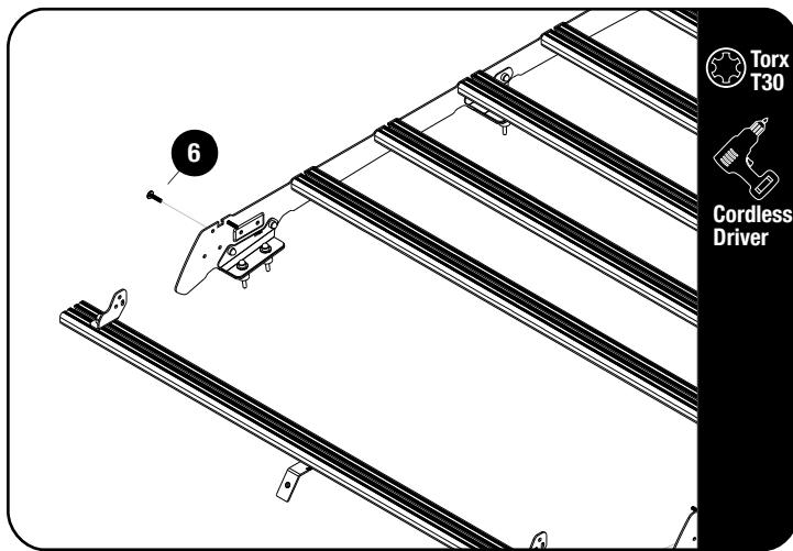
Secure assembly 2.2 to the front two top holes on the foot rails using the fasteners supplied with KSTH002.
